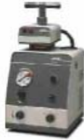
Figure 2: LECO PR-25 mounting press
