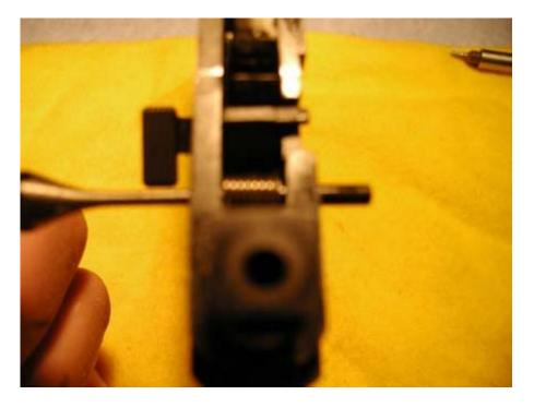
With that out of the way, the sear pin needs to be removed. On most pistols I have been in, it is peened very slightly on the end that sticks out through the safety click plate, and most have the frame staked slightly on the right side. I have a small awl and a very light hammer for this. The pin comes out by tapping the smaller end that sticks through the click plate. This end is almost hidden by the safety lever. See the picture below:
