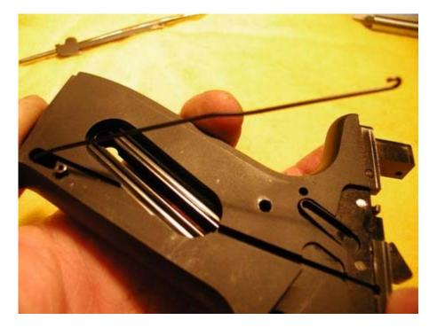
On the left side, the slide stop will be loose, and will be easy to lift out. Note how the small hook on the spring goes through the slide stop in the picture below. If the end of the spring misses the tiny hole in the slide release button, the slide may fail to lock open on the last round, or fail to drop out of the way after inserting a loaded mag.:
