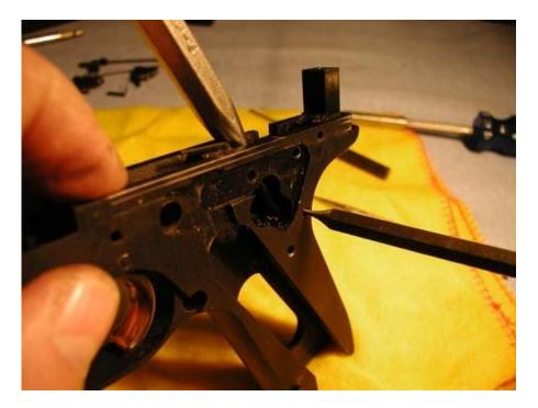
Now the hammer pin can be pushed out from right to left without removing the hairpinshaped slide stop spring:
