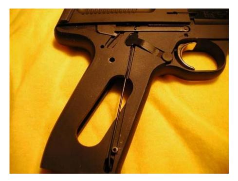
Lift the loose parts off of the grip frame, pull the disconnector spring out and lift the disconnector. Turning the pistol over will dump the mag button. Here's a shot of the disconnector being lifted off with a dental pick:
