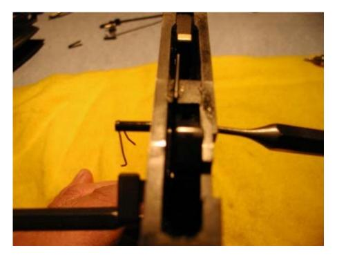
The safety lever rotates for removal and reinsertion. Absolutely no force is required. The original owner of my first Buck Mark didn't understand this concept, and I was never able to get the safety to operate smoothly. The picture below shows approximately how far the safety needs to be rotated for easy removal:
