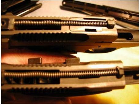
If it is an older one, the slide will pretty much just lift off at this point. Unless you're missing the "C" clip retainer for the slide return spring, no parts will fly off.
