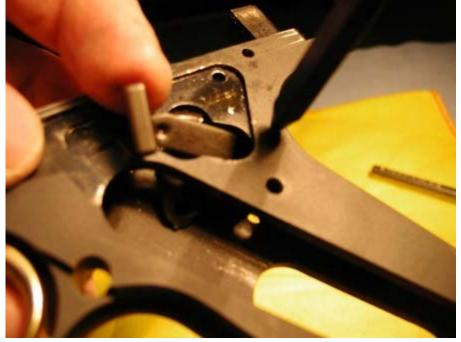
If you want to remove the trigger, the pins should be driven left-to-right. Start with the top pin first. Note that on reinstallation, the depth that this pin is driven in is important. Not far enough and it will drag on the grip. Too much, and it may allow the disconnector to slip off, or it could act as a crossbolt safety by sticking so far to the left that it goes into the hole the factory left for the punch. See photo:
