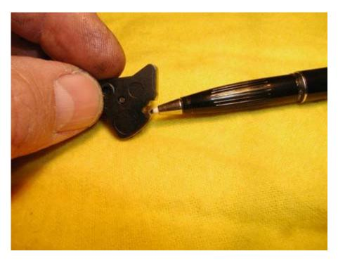
Here's the part of the sear I polished. Again, it is important to simply polish, and not change the shapes or angles of the parts:
