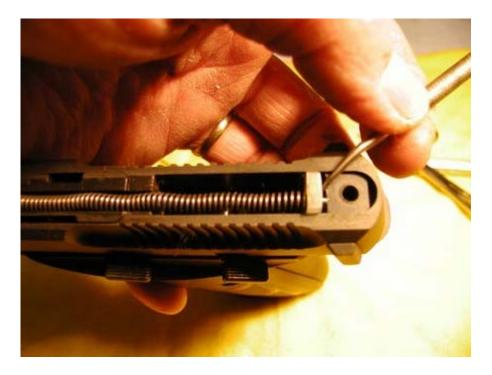
To remove the plastic firing pin guide, use a dental pick to get under it and pry it up and out. There's space between the plastic and the slide to work the hook of a dental pick in below the plastic housing. The housing needs to come straight up so it doesn't bind. So don't try to get it out without moving the pick to the front and rear to keep it even on the way out.) Here's a shot of that:
