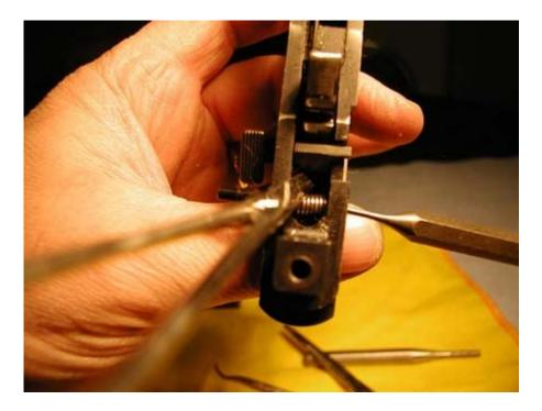
The sear pin is sometimes difficult to get through the safety click plate. One thing I do is work a small pick around in the sear pin hole to get the slightest amount of clearance. For reassembly, I also made a tool from a cheap pair of pliers. I ground most of it away to form a sort of pincher
