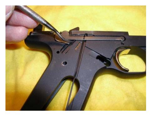
When the disconnector is raised a bit, it can be unhooked from the mag safety link. The link itself can be easily removed by using a mag to depress the spring plunger that the lower end of the mag link engages:
