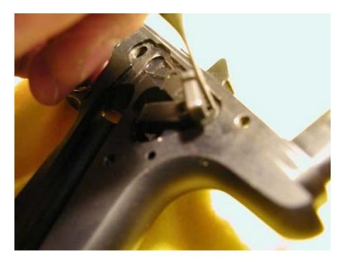
After the pin is pushed in slightly, you can slide the safety click plate forward and off, by gently lifting the front of the click plate off of the hammer pin, and sliding it toward the front of the gun as shown below:
