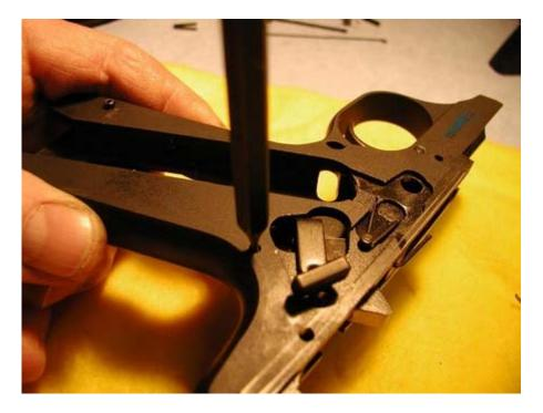
If you wish to remove the mainspring and plunger, simply use another punch as shown in the photo below to depress the plunger. The punch in the picture that is sticking up is lined up in the cupped end of the plunger. It takes quite a bit of force to depress the plunger so the first punch can be removed. "Don't shoot your eye out, kid".
