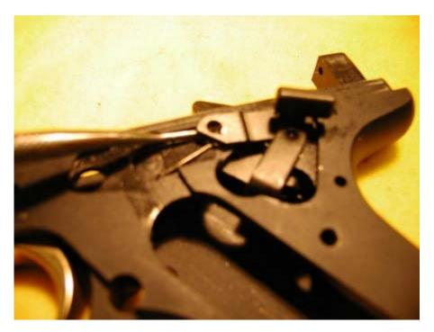
Next you'll need to temporarily lock the mainspring down. Pull the hammer back while having a small punch ready to push through the hole as shown in the picture below. The
